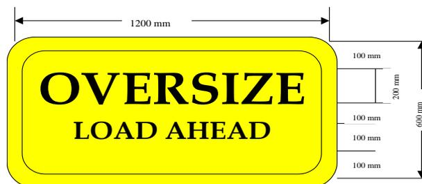
Figure 1: example of a warning sign for a pilot vehicle
